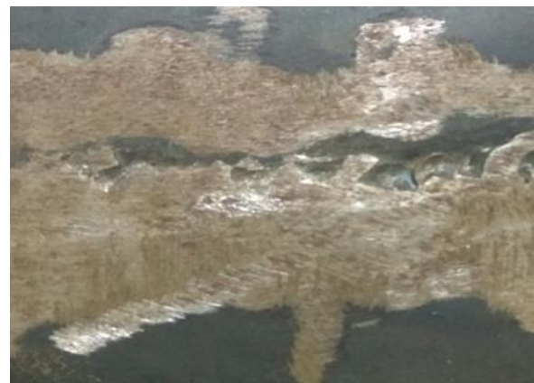
Fig.4 Gas welded steel sheet (Hot & Cold Rolled together)
